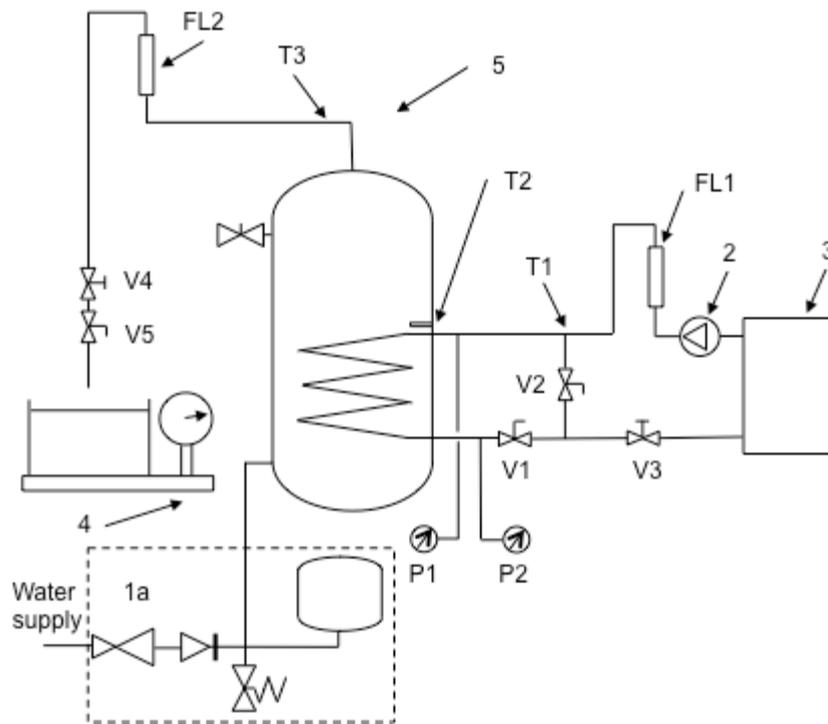
**Figure A2 Apparatus example for vented cylinders**
